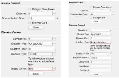
Figure 8-26 Access Control and Elevator Configuration
